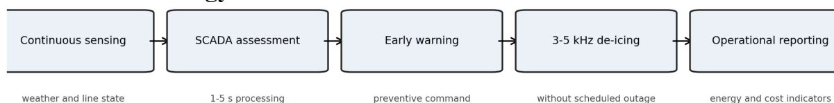
Figure 1. Implemented monitoring, decision, and high-frequency de-icing workflow.
